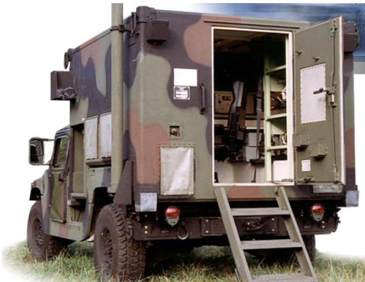
*Figure #6 Military shelter utilizing conductive rubber EMI/RFI gasketing on the perimeter of the door.*
